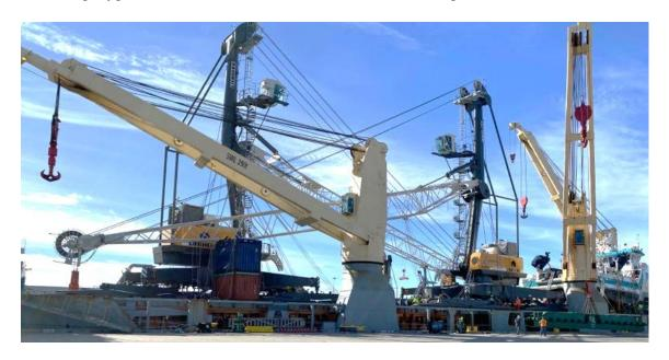
The new crane design has been optimized for ships in the Post-Panamax class. The crane series raises and lowers loads at up to 120 meters per minute and has a maximum load capacity of 124 tons and handles up to 38 containers per hour with its hybrid drive. The crane is also suitable for the efficient handling of bulk cargoes, as well as the safe transportation of general cargoes.
